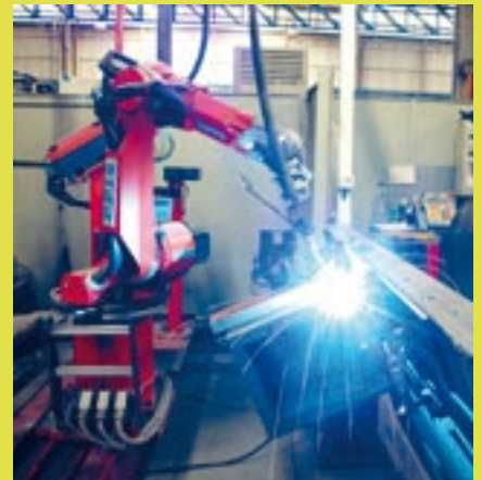
Robot soldadura REIS Welding robot REIS
